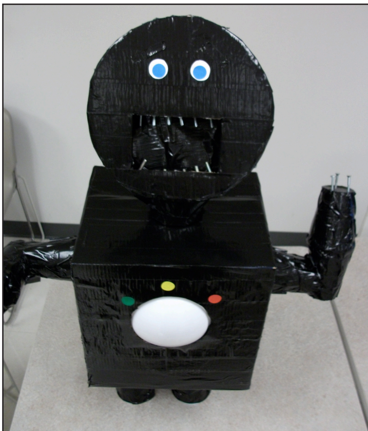
Prototype robot, 31 inches tall, constructed from cardboard, plastic cups, duct tape, sticks, screws, and a push-on light. According to the student designers, if this were a working robot, it would gobble up garbage.
